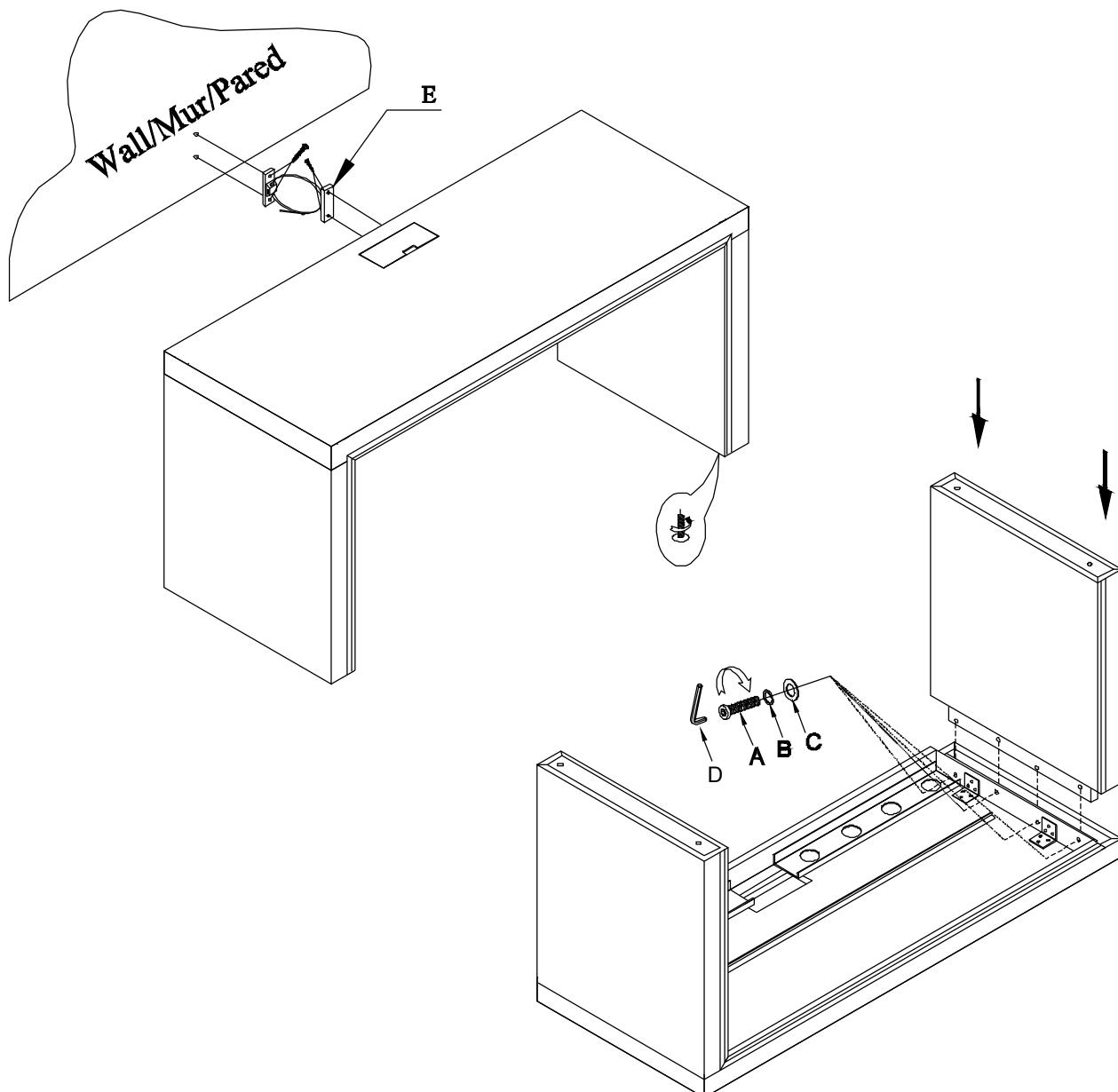
Adjust levelers if needed, to level case on uneven floor
