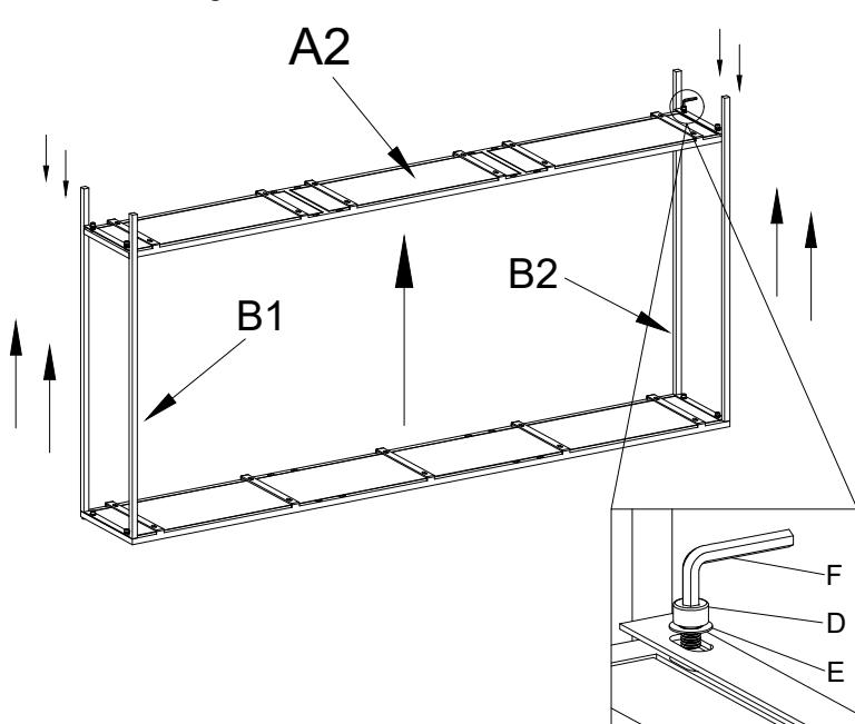
STEP 3. Now assemble the remaining Legs, tighten the bolts for all the legs.
