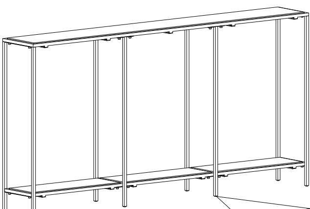
NOTE- Leveller are provided at bottom to balance the product on uneven surface.
