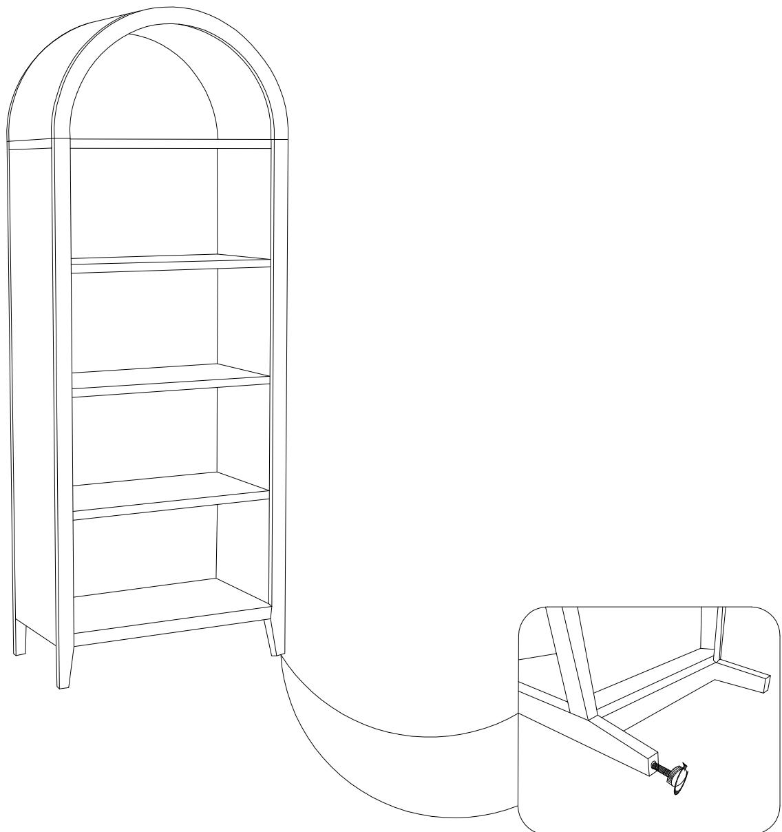
Leveller are provided at the bottom to the balance on uneven surface
