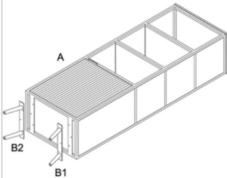
lay down the cabinet on the floor. Align the iron legs with holes on the bottom of the cabinet. (as shown in figure above).
