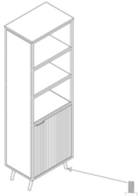
Leveler are provided at the bottom to balance the product on uneven surface
